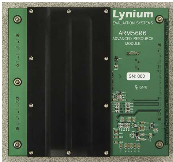
Figure 1. ARM5606 Daughtercard Provides Six High-Resolution, High-Stability DC + AC Voltage Sources.
